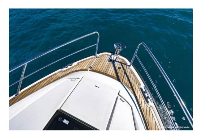
In the stern, the side-decks widen into an area occupied by a large chain locker which also hides an anchor windlass; the anchor (in this case a beautiful Ultra Marine stainless steel one) is placed in view in its bow; for safety and practicality purposes, the stainless steel rail is interrupted at the sides of the bow to allow easy passage to and from the ground.
