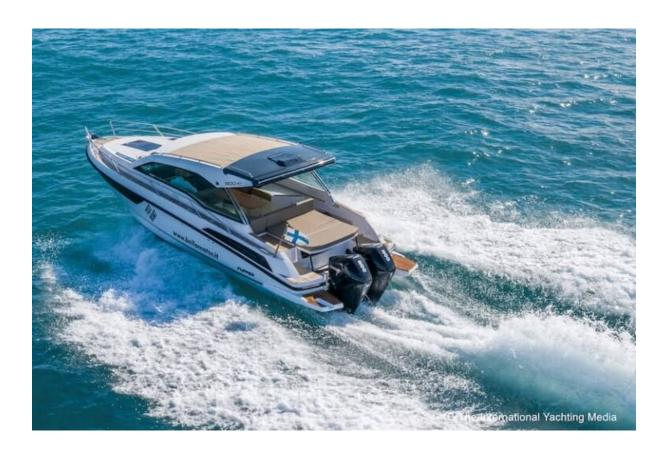
The twin 200HP outboards are more than enough to deliver considerable performance, with a top speed of 38 knots and powerful acceleration. Resulting from a right installed power/waterlines and weight/mass distribution ratio, fuel consumption is rather low: at a cruising speed of 20 knots, the engines use less than 50 l/h.
