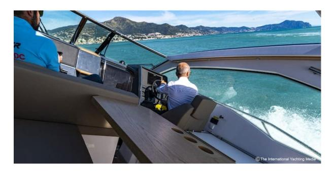
The almost full-beam cockpit results into rather narrow side-decks yet made safe by the abundant presence of handrails. The most comfortable access, however, is offered by the central section of the windscreen and the three steps (obviously covered with solid teak) integrated into the deckhouse structure.
