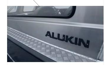
All boats are surface treated with a SEALsystem, a patented chemically bonded surface passivation developed specifically tailored to our boats.
