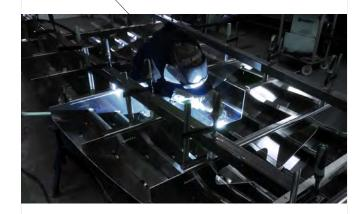
All the hull joints are fully welded from the inside and outside, a solid craft. The material we use in ALUKIN's boats has the strongest alloy for marine use.
