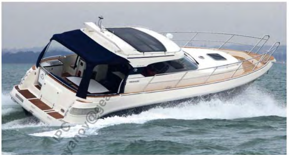
Thanks to the hardtop and the awning, this cruiser almost gains the protection of a wheelhouse
