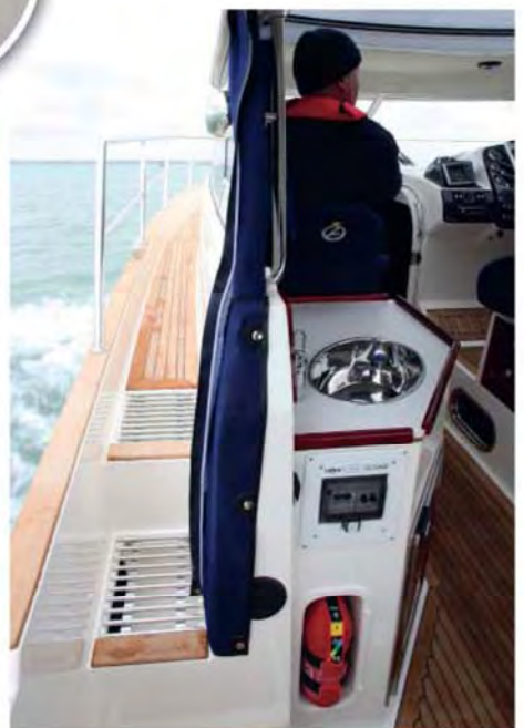
Large scuppers are incorporated into the side decks
